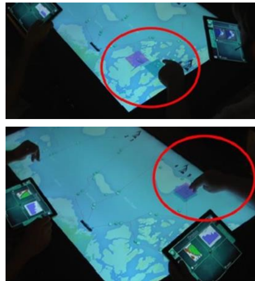
Figure 4. (top) In TILT, SS points at a location where he needs LS to move his ROI, (bottom) In TOUCH, SS uses “flexible ownership” feature to drive LS’s ROI to desired location.
