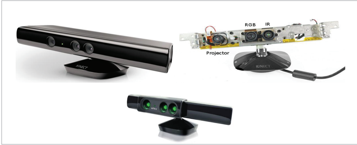
Figure 3: External (top left image) and internal (top right image) views of the Kinect sensor and its zoom lens kit (bottom image) [6].
