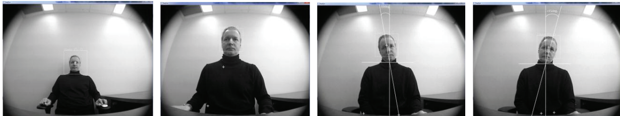
Figure 13: Face detection limits at distance d from the Kinect sensor and at head angle \alpha parallel to the sensor plane.
