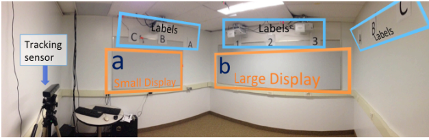
Figure 5. Laboratory setup for the improved study design. Labels were attached to the walls to better simulate signage, with a grid layout for a less straight-forward navigation. A Microsoft Kinect was used at the back of the room to capture the silhouette of the participant and measure depth.
